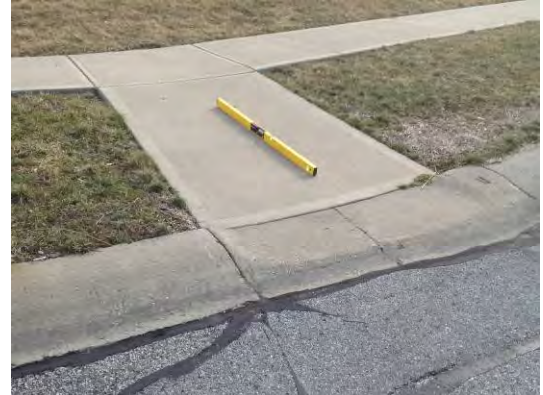
Example of running slope measurement
